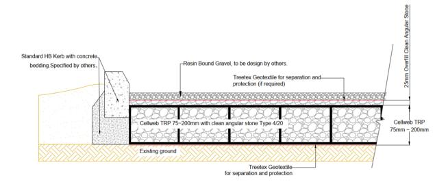
Please provide more details around 'the sub base' generally a CCS does not require a sub base and the CCS laid directly onto the geotextile. If this is in error then please remove and update.
